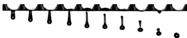
Fig. 3. An illustrative sequence of DOD inkjet drop formation.
